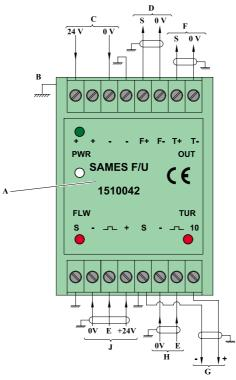
Α Frequency-to-voltage converter, P/N 1510042 В Earthing braid 20 x 2 С Converter power supply D 0 - 10 V output - paint flow F 0 - 10 V output - turbine speed G 0 - 10 V / 10 mA output available for power supply for potentiometer, PLC, etc. Н Microphone signal J Flowmeter signal
